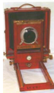
—1902 Box Camera SCHS Collection from Mrs. B Dixon Conrad. Mahogany box with bellows and brass fittings.
